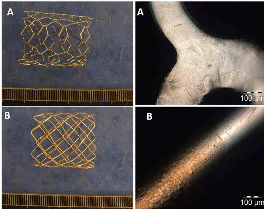
**FIGURE 4** Macroscopic and stereomicroscopic images of stents after 3 month corrosion test. \*A = AN; B = CP. Note: no pitting observed macro- or microscopically [Color figure can be viewed at [wileyonlinelibrary.com](http://wileyonlinelibrary.com)]
