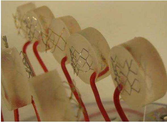
**FIGURE 2** Galvanic corrosion test. Applied samples for galvanic corrosion test (see text). The samples were connected with a copper wire (left) for the electrochemical measurements and mounted in epoxy to isolate the copper material from the test solution [Color figure can be viewed at [wileyonlinelibrary.com](#)]
