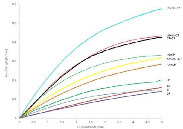
**FIGURE 3** Compression force versus displacement of stents [Color figure can be viewed at [wileyonlinelibrary.com](#)]
